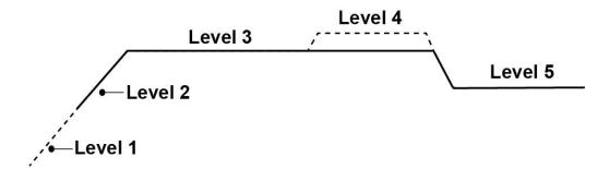
**Soft Charge**- When batteries suffer an over-discharge, the controller will softly ramp the battery voltage up to 10V.
