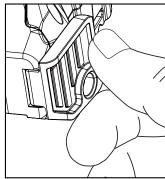
2. With the camera facing open, open the battery compartment cover by sliding the latch to the
