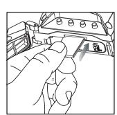
IMPORTANT: Make sure the camera is powered off before removing or installing an SD card.
