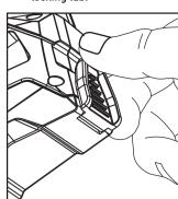
With the camera facing open, open the battery compartment cover by sliding the latch to the
