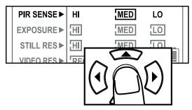
2. Press the left or right navigation button to move to different options. Press the OK button to save the setting.
