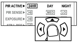
2. Press the left or right navigation button to move to different options. Press the OK button to save the setting.
