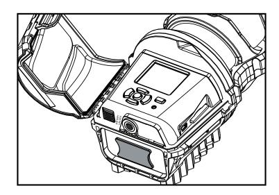
Push the battery latch up to unlock. At the same time grab the battery compartment out.
