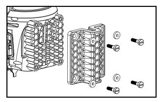
2. Once the camera is attached connect the T-Post bracket to your T-Post.
