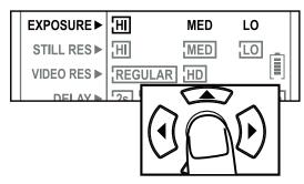
2. Press the left or right navigation button to move to different options. Press the OK button to save the setting.
