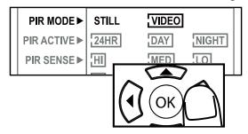
1. Press the OK button while PIR Active is selected. The highlighted option will be blinking.
