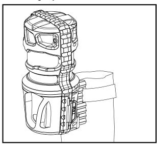
1. When mounting to a T-Post, first attach the T-Post bracket to the camera.
