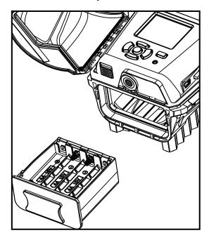
Once the batteries are in the appropriate spot, return battery compartment.
