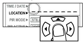
2. Press the UP or DOWN navigation button to go up or down in sequence. Press the OK button or the Left and Right navigation button when the character shown is what you want and move to the next character.
