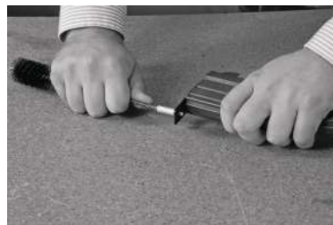
Magazine takedown tool removes butt plates quickly and easily
