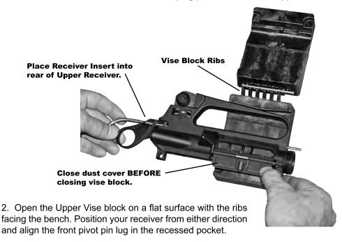
3. Close the Upper Vise Block and inspect for proper positioning. There should be a gap of approximately 1/16" opposite of the hinge. A gap in excess of 1/4" may suggest the upper receiver is not Mil Spec and clamping in a vise may damage the Upper Vise Block. The Wheeler Engineering Delta Series Upper/Pic Rail Vise Block (#156888) will work for these uppers.
