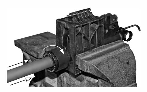
4. Once you have applied the proper barrel nut torque, use the gas tube alignment rod to check for proper barrel nut alignment. Make necessary adjustments until the gas tube alignment rod passes through the receiver and into the barrel nut freely.
