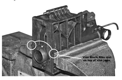
5. Once the Upper Vise Block has been securely clamped into a bench top vise, your upper receiver is ready for all your maintenance needs.
