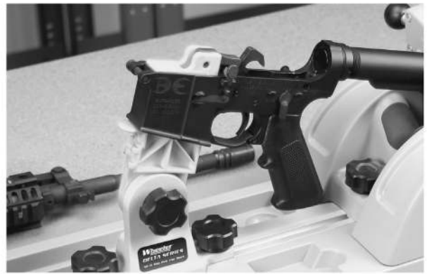
Mag well Vise Block mounted to Best Gun Vise
