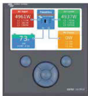
Color Control GX, showing a PV application
