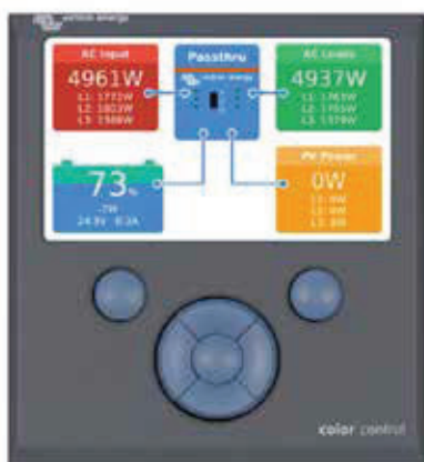
Color Control GX, showing a PV application
