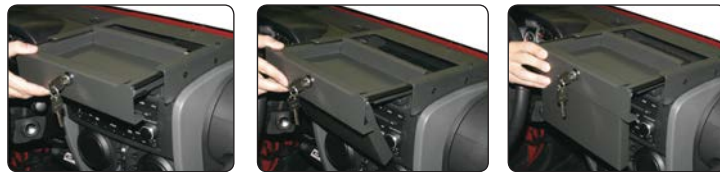
Step 1: Unlock & slide out Step 2: Flip lid down Step 3: Slide in and lock
