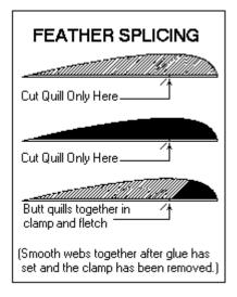
Another method of splicing is to fletch 2 or more sections of "full length" feather pieces, then cut or burn the final shape with a feather burner.
