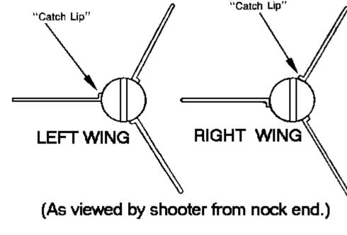
Second method: Hold the forward end of a diecut (pointed end) or full length feather (large end) toward yourself. Look down from the top. Rotate the feather so that its web is horizontal and its natural
