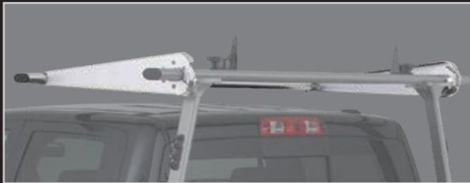
**44000-01, 44000-02 Cantilever Extension** – Protect your truck cab from potential damage carrying long loads, the cantilever provides 32 inches of additional coverage.
