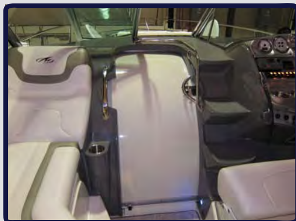
Sliding Cabin Entry Door with Stainless Handle & Flush Latch (Closed View)
