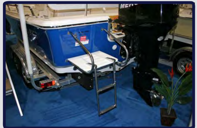
King Starboard (Poly) Dive Platform with Double Step Telescoping Ladder
