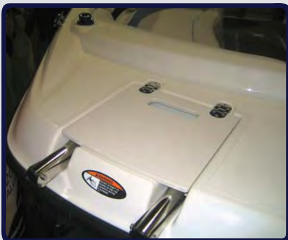
King Starboard (Poly) Anti-Skid Ladder Lid
