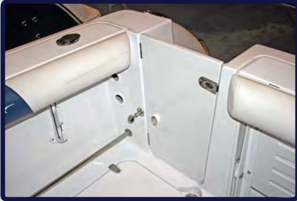
King Starboard (Poly) Transom Door with Magnetic Latch
