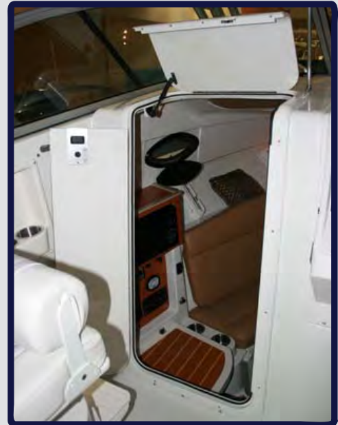
Aluminum Framed Acrylic Cabin Entry Door with Hatch (Open View)
