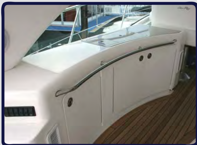
Bent Acrylic Doors with Corian Countertop Inserts
