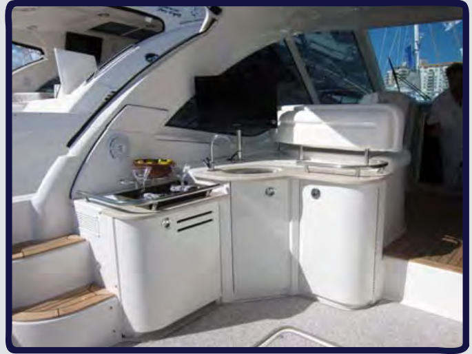
Bent Acrylic Wetbar Doors and Corian Countertop
