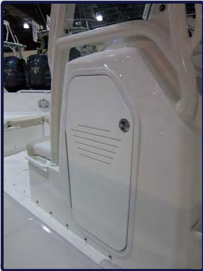
King Starboard (Poly) Console Door with Powder Coated Aluminum Frame and Vented Louvers
