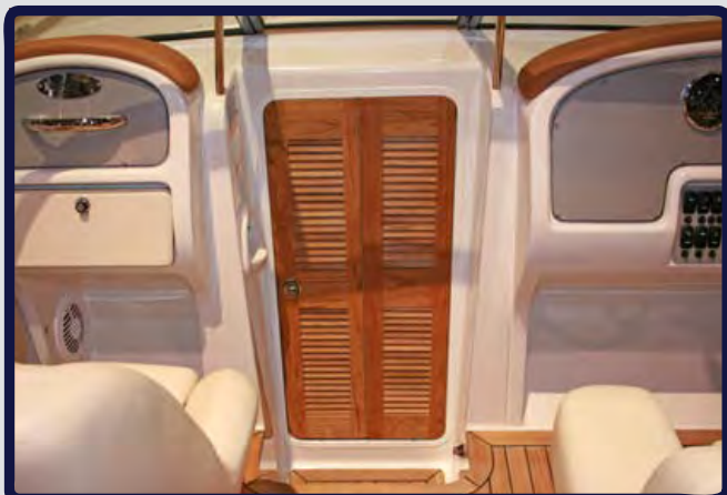
Teak Louvered Cabin Entry Door with Powder Coated Frame
