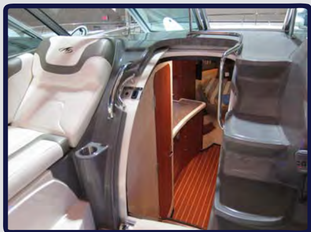
Sliding Cabin Entry Door with Stainless Handle & Flush Latch (Open View)
