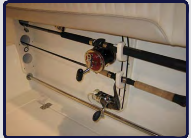
Load and Lock Rod Holders and Rod Holder Tube Assembly
