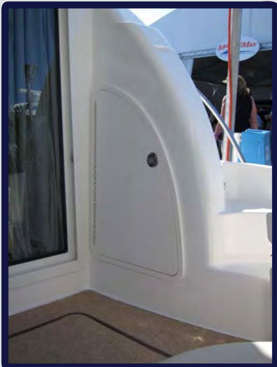
King Starboard (Poly) Wing Panel Door Custom Shaped to Maximize Usable Space
