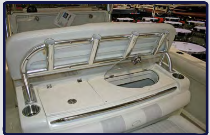
Starboard (Poly) Baitwell Lid Assembly and Sink Cover Combo with Acrylic Baitwell Lid
