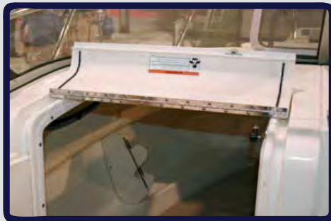
Acrylic Hatch with Weather Resistant Seal
