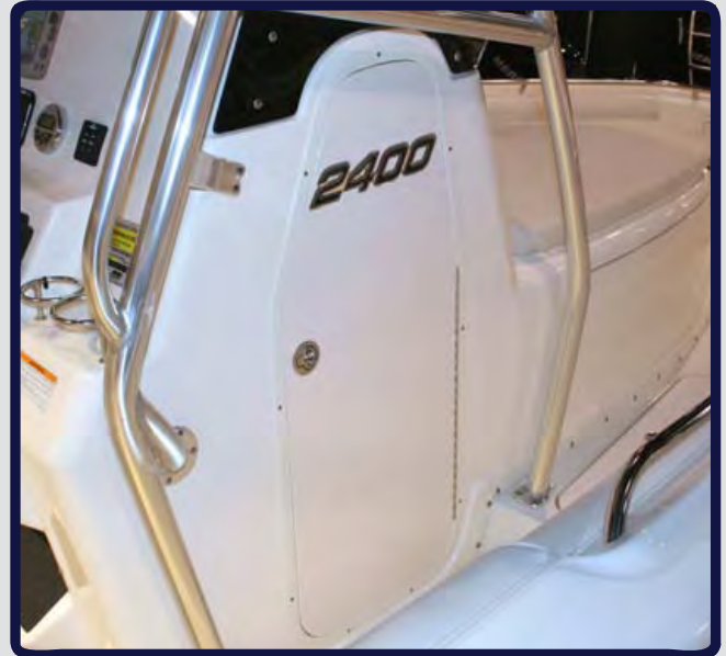
Acrylic Console Door with Powder Coated Aluminum Frame
