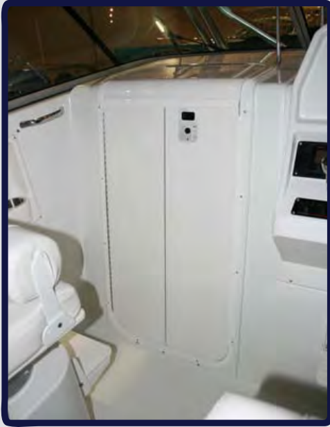
Aluminum Framed Acrylic Cabin Entry Door with Hatch (Closed View)
