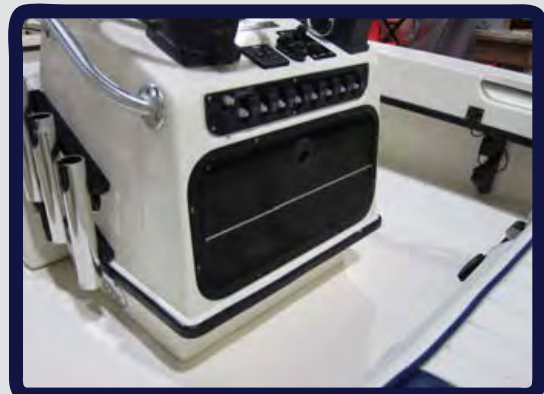
Powder Coated Aluminum Framed Removable Drop-in Acrylic Door
