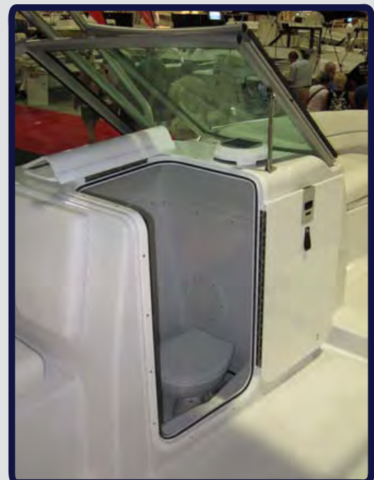
Radius Corner Powder Coated Aluminum Frame with Acrylic Door and Bent Hatch
