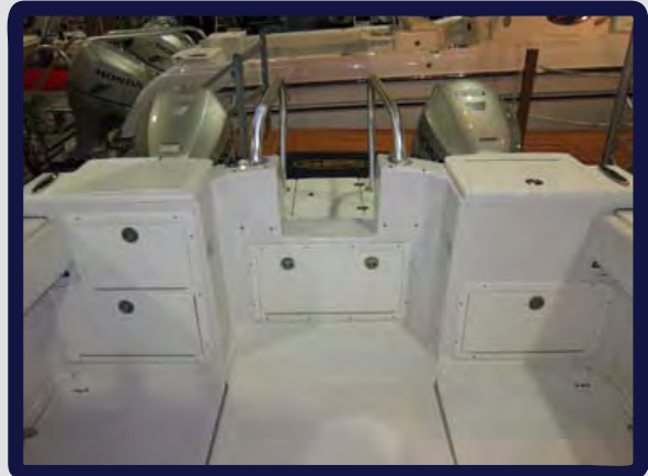
King Starboard (Poly) Access Doors and Tackle Storage Units
