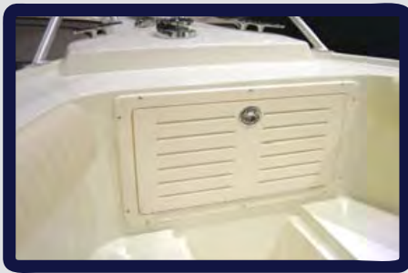
King Starboard (Poly) Anchor Locker Door with Vented Louvers
