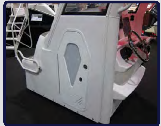
King Starboard Console Door with Frosted Acrylic Window Panel and Vented Louvers
