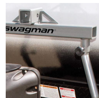
■ RECEIVER CAN BE RAISED OVER PROPANE TANKS
