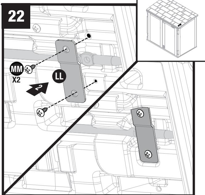
Attach prop rod bracket (LL) using two screws (MM).
