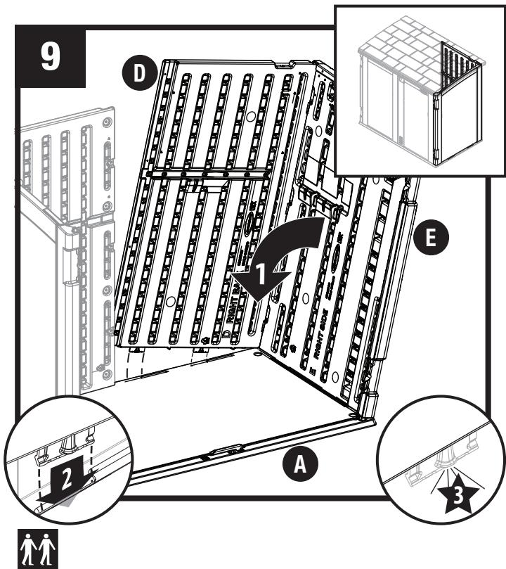
Tilt right back panel (D) and right side panel (E) back into the upright position (lowering the right back panel tabs into the slots of floor (A)). The right back panel tabs will 'snap' into place when in correct position.
