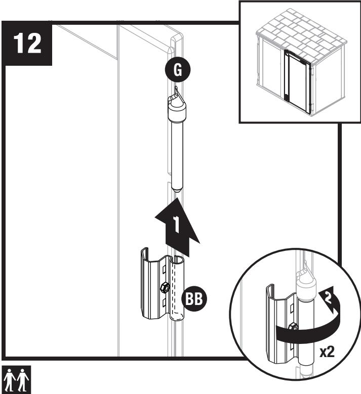
Stand right door (G) upright with two hinge mounts facing right. Slide one metal hinge plate (BB) onto each hinge mount. Rotate metal hinge plates to open position.
