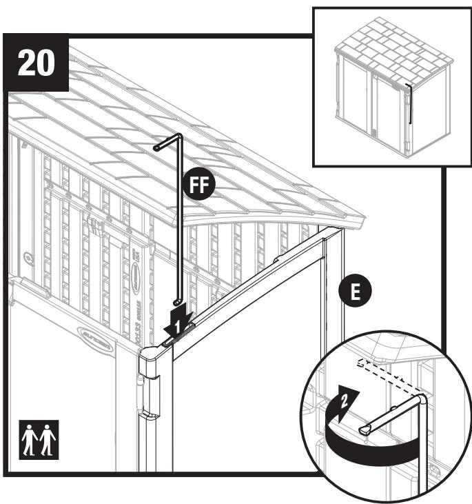
Insert prop rod (FF) into right side panel (E) and turn clockwise.
