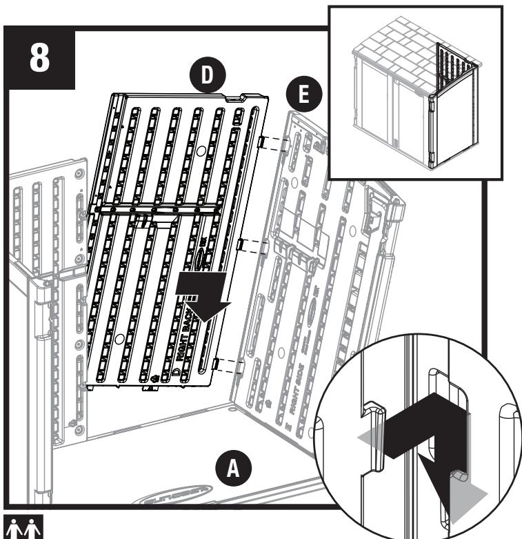
At an angle, align tabs on side of right back panel (D) with slots on right side panel (E). Move right back panel in and down into right side panel to secure.
