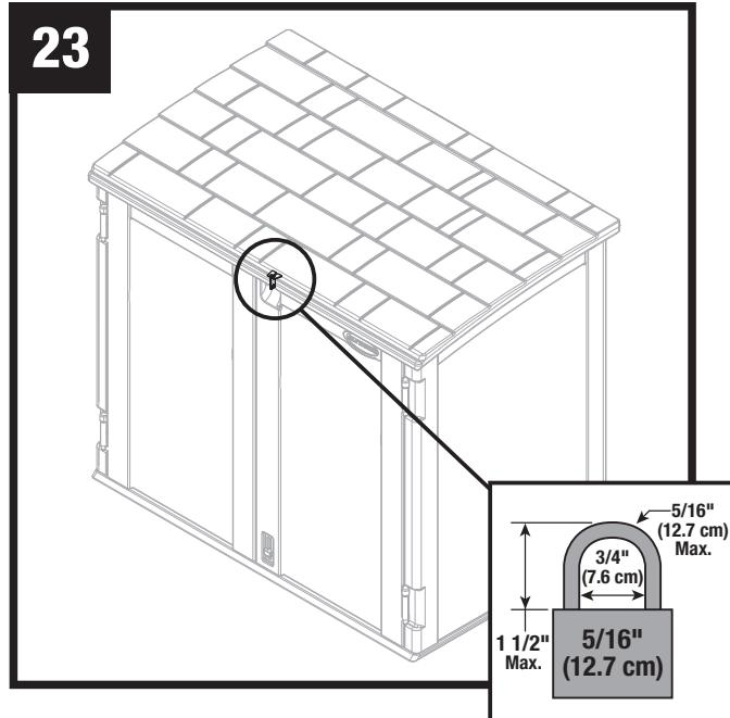
With roof closed, attach a 5/16" lock (not provided) to lock hasp (GG) to properly secure shed.
