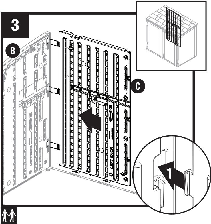
Align tabs on edge of left back panel (C) and insert into slots on the left side panel (B).
