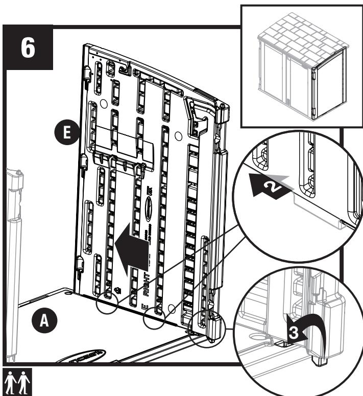
Lock side panel (E) by sliding panel toward rear of floor panel (front corner tab will slide over floor and into position).
