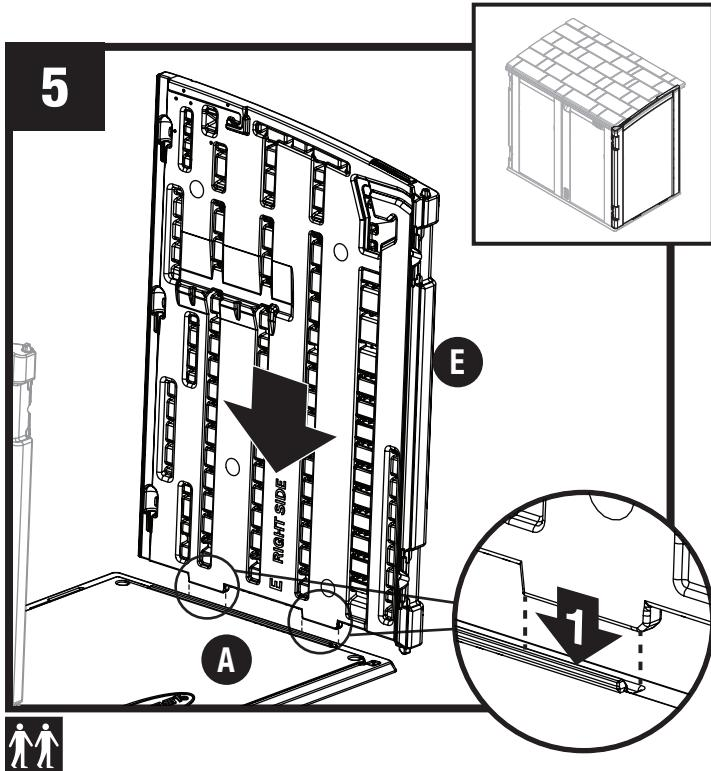
Align tabs on bottom of right side panel (E) with slots on floor (A). Lower panel into slots.
