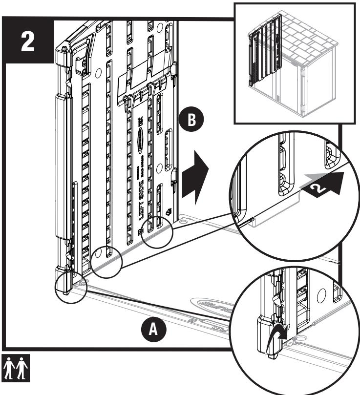
Lock side panel (B) by sliding panel toward rear of floor panel (front corner tab will slide over floor and into position).
