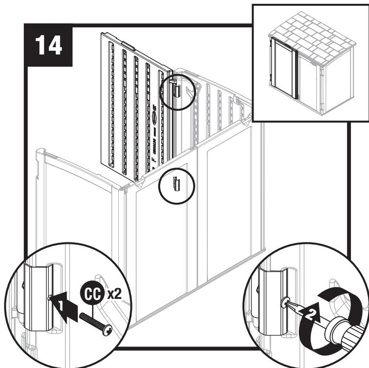
Secure each door hinge with one screw (CC).
