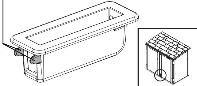
Insert door latch housing (EE) into bottom right door (G) and snap into place. Insert door latch (II) into door latch housing. Push latch pin down so it is fully seated in latch housing. Push down with force until you hear a snap. Slide latch up and down to confirm it slides properly.
