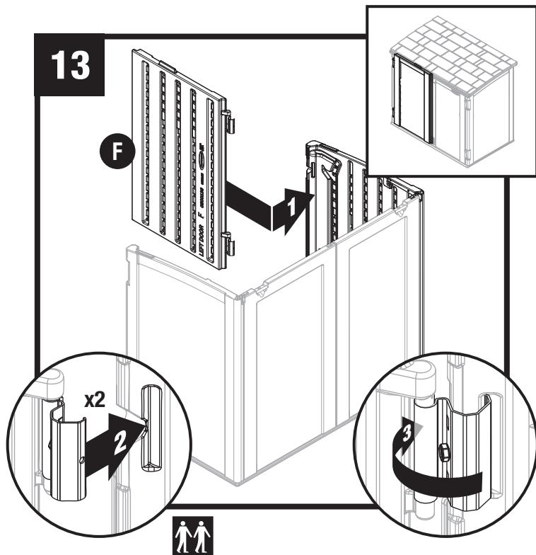
Slide one metal hinge plate over each hinge receptacle on inside of left side panel.
