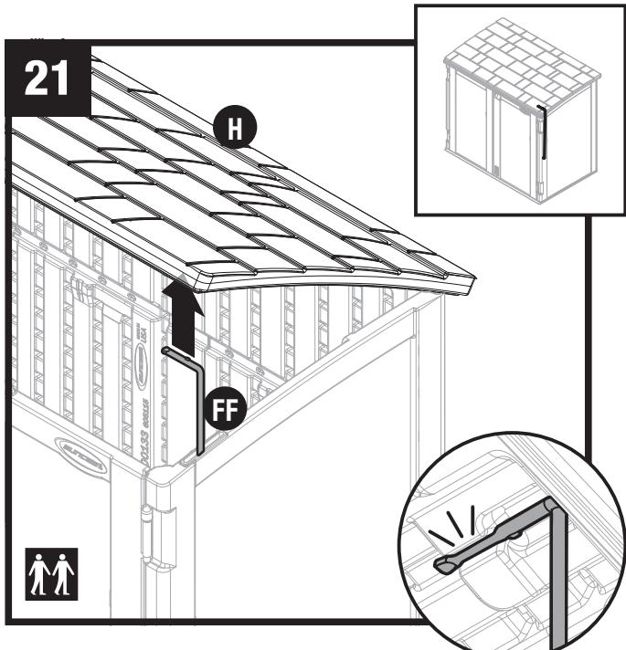
Lift prop rod (FF) up and attach to bottom of roof (H).
