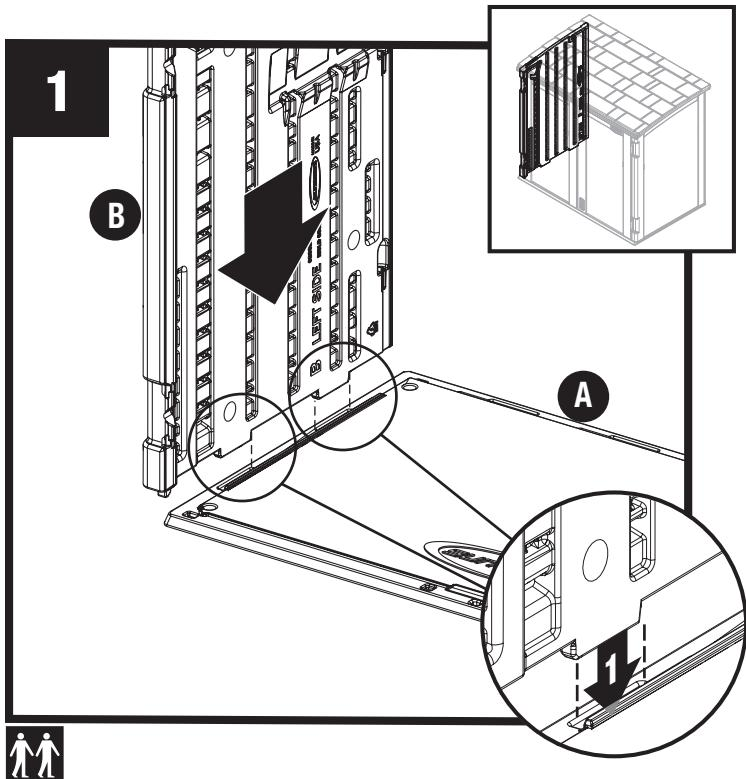
Align tabs on bottom of left side panel (B) with slots on floor (A). Lower panel into slots.
