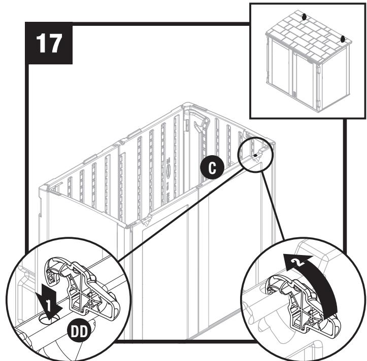
Insert one hinge half (DD) into left back panel (C) and rotate up.
