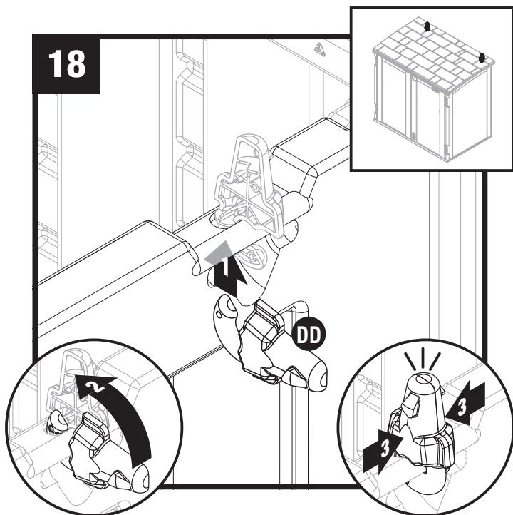
Insert second hinge half (DD) and rotate up. Push the two hinge halves together.
