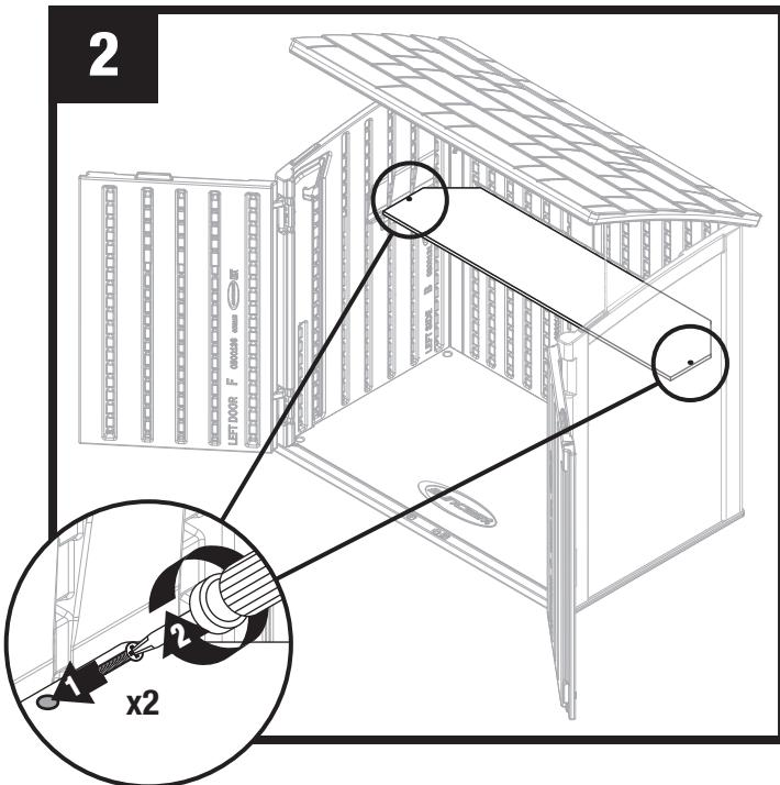
To secure shelf, insert one #8 x 1.25" drywall screw (not provided) through each pilot hole and into side panels.
