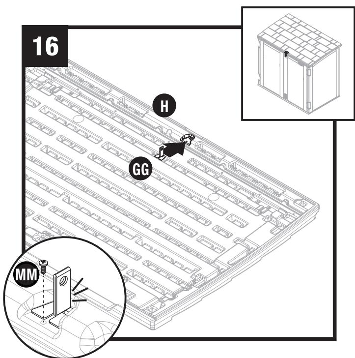
Attach lock hasp (GG) to bottom of roof (H). Secure with one screw (MM).
