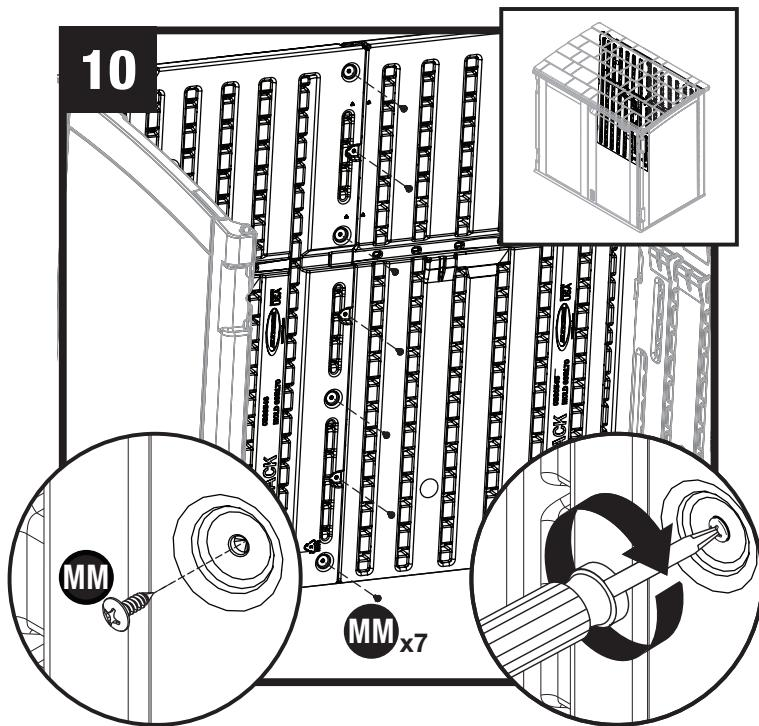
Secure back panels (C, D) together with seven screws (MM).
