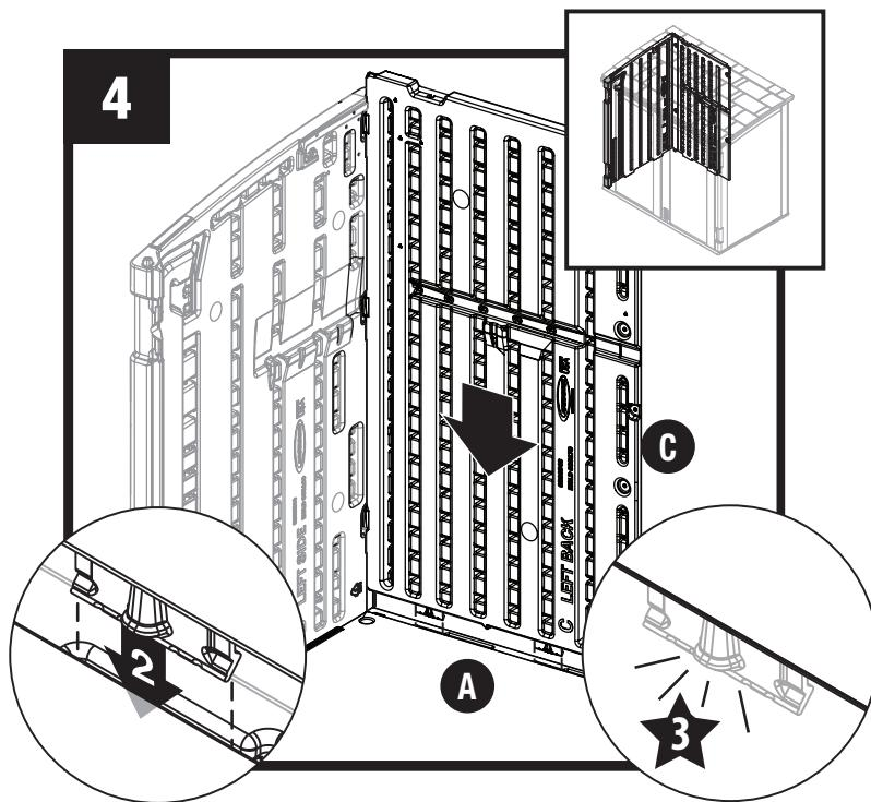
Lower the left back panel (C) tabs into the slots of floor (A), and snap into place when in the correct position.
