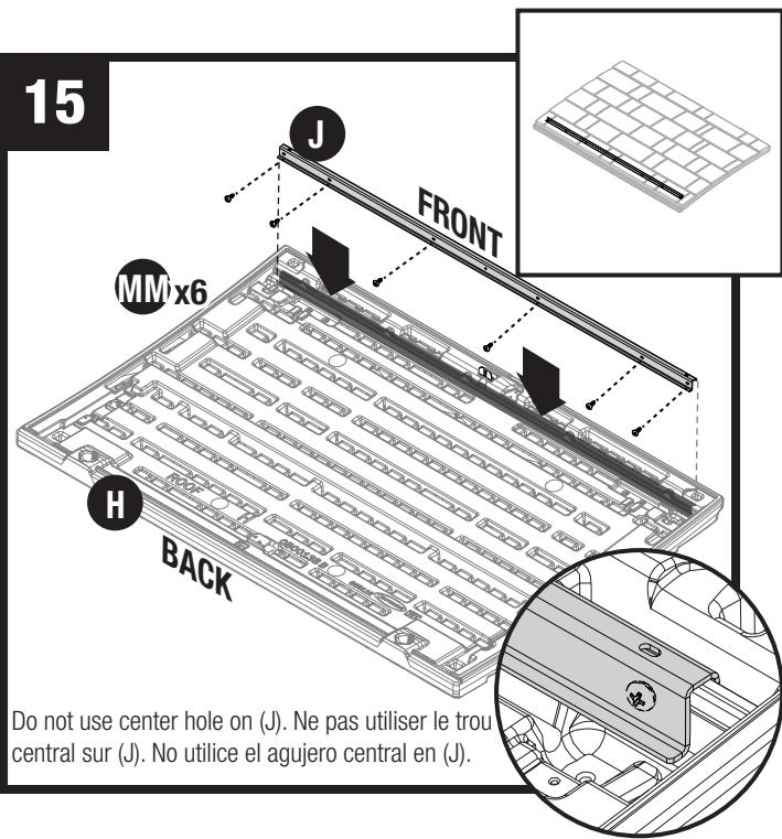
Lower support bracket (J) into position on lid (H). Attach through pre-drilled holes using six screws (MM). There are no pre-drilled holes on the lid. Use force when starting to drive self-taping screws. Once the screw pierces the plastic it will drive easier.
