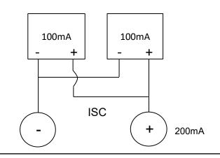
Our panels have outputs that meet or exceed the rated specifications. Panels are tested using VOC: Voltage Open Circuit, ISC: Current Short Circuit. Test simulation, using 1 Colorado sun at high noon at 28°C.
