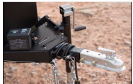
2" front receiver accepts multi-axis articulation couplers
