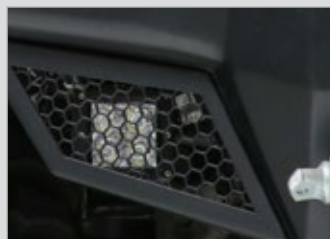
Removable mesh panels include provisions for 3"x3" LED cube lights
