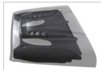
8.7mm thick underbody insulation mat
