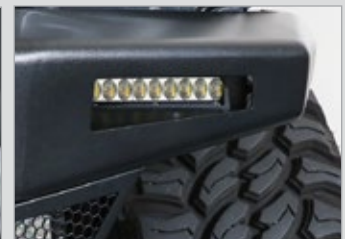
Front bumper includes 21" and (2) 6" LED light bars. Rear includes (2) 6" LED light bars
