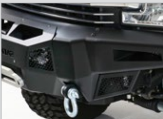
1/8" steel with a 3/4" radius construction provides performance and protection
