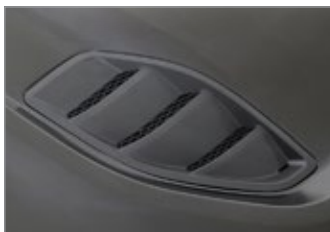
Vent hot gasses out of engine bay
