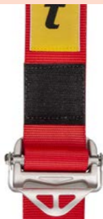
O7 Hook and loop fastener on upper shoulder belt.
