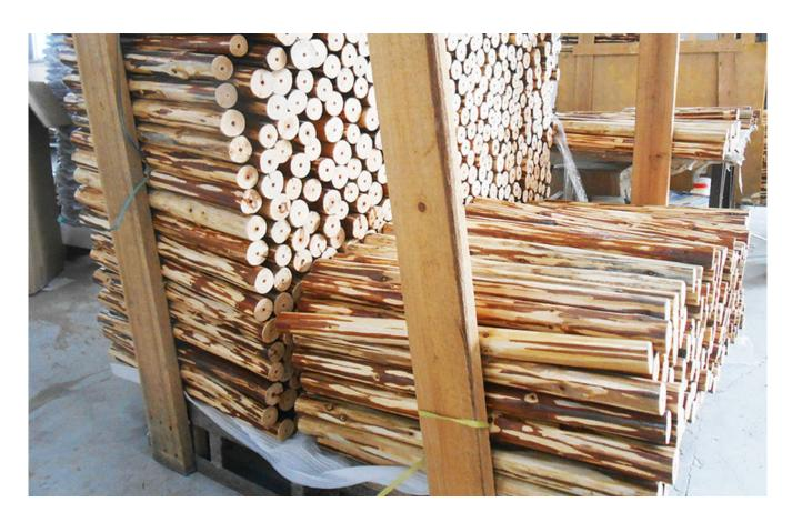
Our wood is hand selected using only the highest grade of pine conducive to our manufacturing process. The selected wood is air-dried for 8 to 12 months then kiln dried for another 60 days. The logs are then tested with the state-of-the-art moisture meter to ensure optimum levels. Only after this lengthy, precise process can our logs be transformed into beautiful furnishings.
