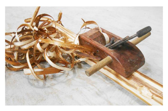
The construction begins only after the wood has been approved for final production. We start by hand-stripping the bark of each log, skip-peeling. This process is completely done by hand with a drawknife so no two logs are alike. After each log has been crafted, the ends are fitted with quarter inch threads that require bolt fastening. Other joints are pre-assembled and fitted twice then expansion glue is applied for the tightest fit possible.
