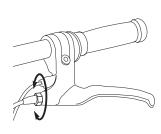
**1** To adjust the brake cable wire, thread the brake lever adjuster in or out 1/4 to 1/2 turn until the desired cable tension is attained.
