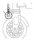
**3** If the brake is too tight or too loose, use a 8mm open wrench and a 3mm allen wrench to make adjustments as needed.
