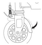
**2** Squeeze the hand lever to test the brake to make sure it is working properly. The front fender should clamp down and rub against the front wheel. If brake is not working properly, proceed to the next step.
