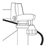
**3** Slide the handlebar stem down into the front fork until it fits snuggly into the lock nut on the headset.
