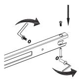
**1** Remove black plastic protector at the end of the frame. Using two 5mm hexagonal wrenches, remove the two hexagonal bolts and the two coupling bolts from the frame.
