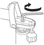
**4** Using a 5mm hexagonal key wrench to tighten the stem bolt. The stem bolt is properly tightened when the handlebars cannot be twisted out of alignment with the front wheel. Make sure the handelbars are in line with the front wheel before tighten stem bolt all the way.
