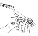
**2** Align parallel to the fork and tighten the bolts using a 6mm Allen wrench. When properly tightened, the handlebars should not move forward or back.
