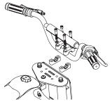
**1** Place the handlebars in the handlebar clamps.
