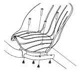
**2** Align the four (4) holes in seat with the four (4) holes in frame. Insert the coupling bolts through the top and bottom of the frame.
