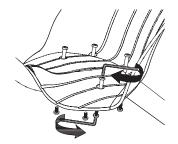
**3** Tighten the coupling bolts using two (2) 5 mm Allen wrenches.
