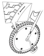
**2** Insert the wheel assembly into the front fork and align holes. When installing the wheel, make sure the letter **"F" and arrow** (located on the side of the wheel) are facing the direction as shown above.
