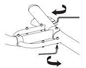
2 Insert the rear frame into the frame assembly. Securely tighten the coupling bolt on the rear frame using two (2) 5 mm Allen
