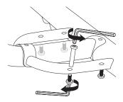
**1** Using two (2) 5 mm Allen wrenches, remove the four (4) coupling bolts from the frame.
