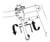
3 Align the holes on the Spark Handle with the holes on the Spark Bar and tighten the coupling bolts with a 10 mm wrench and a 5 mm Allen wrench.
