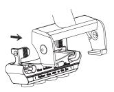
**2** Place new cartridge in back of the bracket making sure to align the slots on the cartridge with the two legs of the bracket. Slide the cartridge forward until you hear a click and the thumb tabs are locked in place.
