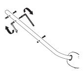
1 Using a 10 mm wrench and a 5 mm Allen wrench, remove the coupling bolts from the Spark Handle.
