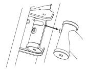
**3** Be sure to properly align the slot on the headtube with the pin on the front fork as shown.
