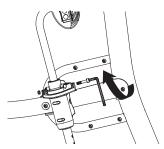
2 Insert the Spark Handle (right side) and the Spark Bar (left side) into the spring mechanism. Align the holes on the Spark Bar with the hole on the spring mechanism and tighten the coupling bolt with a 10 mm wrench and a 5 mm Allen wrench.
