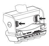
**1** Using your thumbs, press tabs on both sides of the cartridge to release from the bracket. Slide the cartridge away from you and remove from bracket.
