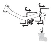
1 Using two (2) 5 mm Allen wrenches, remove the coupling bolt on the end of the frame and discard the plastic insert. Remove the coupling bolt in the middle of the frame.
