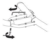
3 Securely tighten the coupling bolt in the middle of the frame using two (2) 5 mm Allen wrenches.
