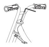
**4** Reinsert the steering bolt and secure with locknut using a 13 mm wrench and a 5 mm Allen wrench.
