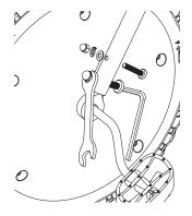
**3** Reinsert the coupling bolts through the front fork and tighten securely.
