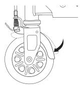
**2** Squeeze the brake lever to test the brake to make sure it is working properly. The front fender should clamp down and rub against the front wheel. If brake is not working properly, proceed to the next step.
