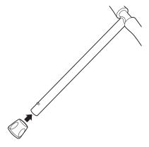
Slide the steering clamp cover onto the T-bar.
