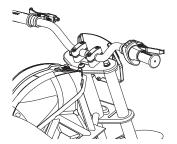
**2** Align with the front fork and tighten the bolts using a 6 mm Allen wrench. When properly tightened, the handlebars should not move forward or backward.
