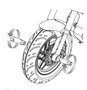
**3** Slide axle bolt through the front fork, spacer and wheel hub. When axle bolt passes through the other side of the wheel hub, add the other spacer, and slide through the front fork. Secure with washer and nut.
