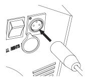
**2** Plug the charger into the charger port. The light on the charger should turn red during charging then back to green when charging is complete.
