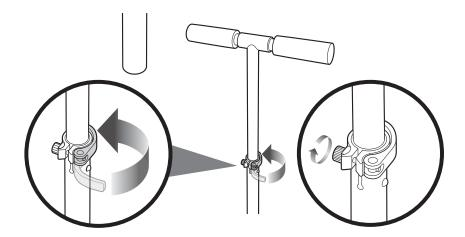
**2** The tension of the quick-release lever can be adjusted by manually tightening or loosening the Allen bolt. Be careful not to over-tighten. You should always be able to open and close the quick-release lever by hand and the T-bar should slide freely when the quick-release is open.
