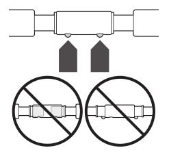
**3** Make certain **BOTH** handlebars are properly locked onto the T-bar.
