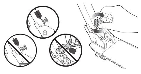
**Note:** To activate the anti-rattle feature twist the knob to the right to tighten. Please note there is no need to over tighten.
