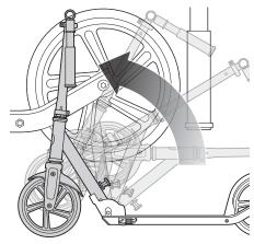
**Note:** The Anti-Rattle knob is spring-loaded and will automatically lock in the upright position when fully upright.
