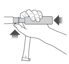
**2** Insert and secure the left and right handlebars by pressing the spring-loaded buttons and inserting them into the T-bar.
