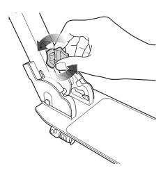
1 To fold scooter you must first deactivate the antirattle feature. Twist the knob left until loose. No need to loosen knob more than one full turn.
