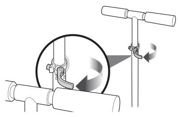
**1** To adjust the height of the handlebars, open the quick-release lever and slide the T-bar to the desired position and resecure the quick release lever to lock into place.
