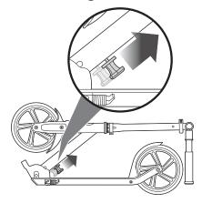
1 To release the folding mechanism, place the scooter on the ground, put one foot on the deck plate and pull the Anti-Rattle knob up.
