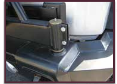
Adjustable, easy swivel hinge with grease fitting.
