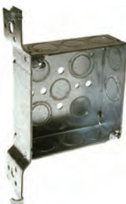
BOX-LOC® "MS" Bracket Positions box on either side of stud. BOX-LOC® (MS) Bracket Box is a snap to install. Place the bracket on the open side of the stud first. Slots in the bracket engage the lip of the stud and actually crimp it as you press the bracket on the stud. Barbed hooks dig into the flat side of the stud, quickly locking it into place.
