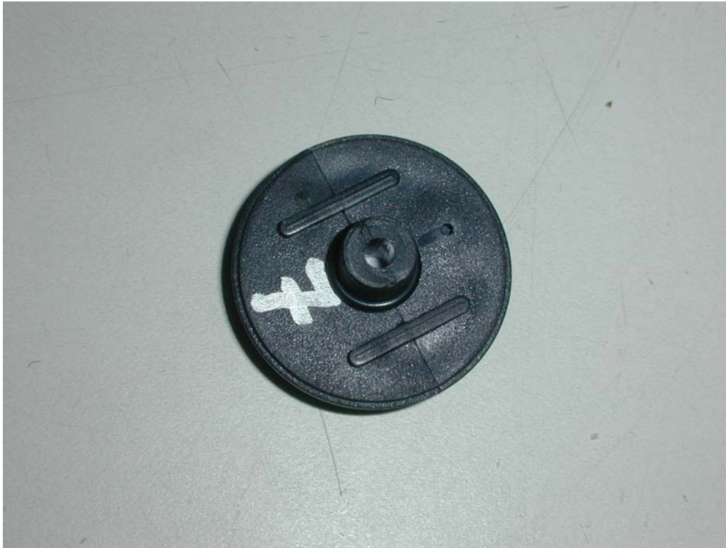
Photograph 4-8: Vent upon completion of the incubation period
