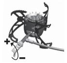
A yellow, flaring flame means that the burner is not hot enough or that you have opened the control valve too far. Start off by closing the control a little. If the flame does not turn blue after
