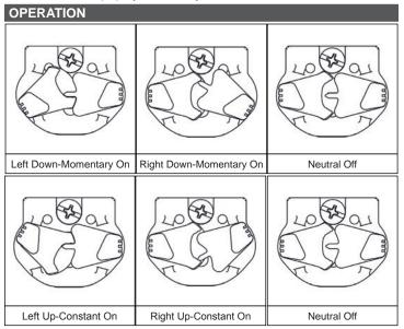
• The TWM uses Dual Dependent Locking Switches.
