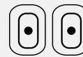
Left Button: Reticle brightness settings and On/Off button Right Button: Dot brightness settings and On/Off button
