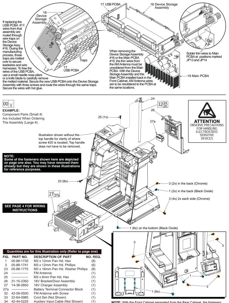
**NOTE:** With the Front Cabinet separated from the Rear Cabinet, the fasteners that are indicated in this illustration must be removed from the Rear Cabinet in order to take out the Charger Assembly #27.
