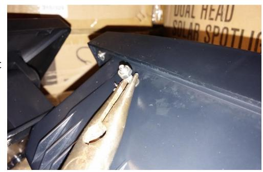
While still holding the bolt with the needle-nose pliers, place one hole of the solar panel over the bolt. The small size of the needle-nose pliers should allow clearance to do this. Continue to maintain your grip on the bolt with the needle-nose pliers.
