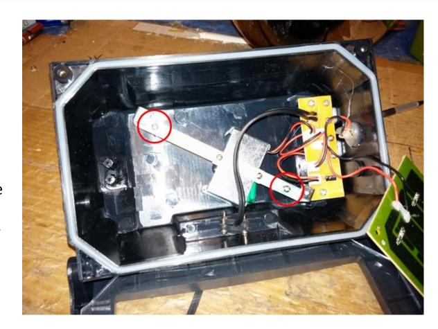
After removing the screws, remove the bracket. This will expose the battery pack. You will see the battery pack is plugged into the control board.
