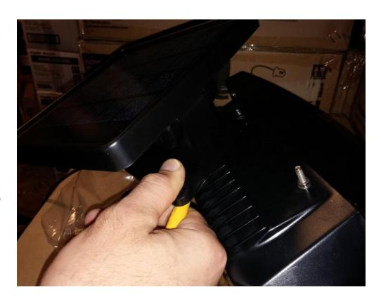
Place the nut back on the bolt and twist it a few times to ensure it is in place, but do not tighten it at this time. You can now let go of the bolt with the needle-nose pliers. It is necessary for the nut to be a little loose so you are able to place the other side of the solar panel.
