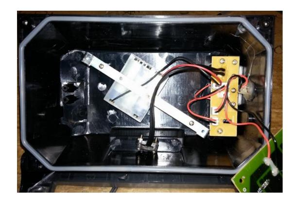
Put the LED Board back in place on the bracket. Use the remaining bolt from when you first removed it, and one the remaining bolt from Step 7 when you removed the battery cover from the bracket.
