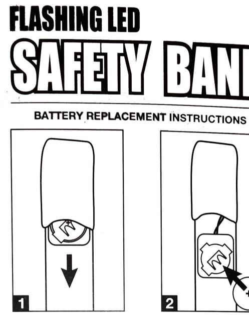
Gently pull battery holder out from beneath the elastic pouch on back.
