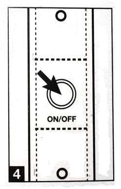
Turn safety band over and press ON/OFF button to turn on flashing lights.
