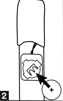
Remove old battery.\* Insert new CR2032 (3V) battery into holder with positive (+) side facing top of holder.
