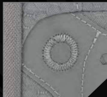
Circular Reinforcement Bartacks
