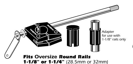
The round rail, quick-disconnect, all angle mounting bracket is made entirely of 18-8 stainless steel and 356 anodized aluminum to endure the most severe marine environment. Fits any angle railing and detaches quickly for storage without tools, leaving no hardware on the rail.
