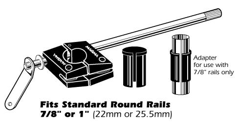
The round rail, quick-disconnect, all angle mounting bracket is made entirely of 18-8 stainless steel and 356 anodized aluminum to endure the most severe marine environment. Fits any angle railing and detaches quickly for storage without tools, leaving no hardware on the rail.
