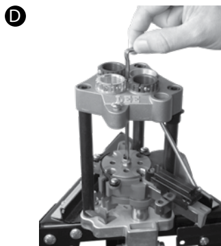
With the carrier at the bottom of the stroke (handle up), install index rod.
