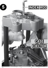
Remove index rod and case ejector.
