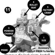
Remove die lock rings. Install dies according to instructions.
