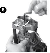
Raise carrier to the mid-stroke position, install shell plate, lightly tighten clockwise with '4" hex head wrench
