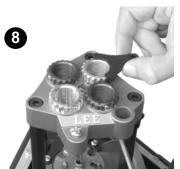
Install spline drive breech lock bushing. Snug with die wrench.
