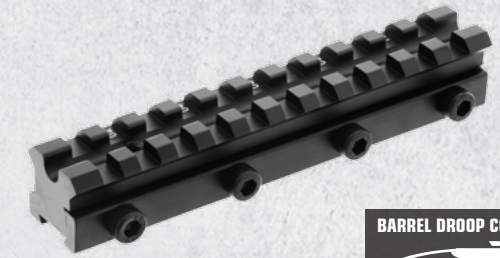
MNT-DNT06 Compensation Mount for T06 Tigger Equipped RWS Diana Air Rifles • Precision Machined from Aircraft Aluminum with a Matte Black Finish • Compensation to Bring the POI (Point Of Impact) Up 10 Inches at 30 Yards
