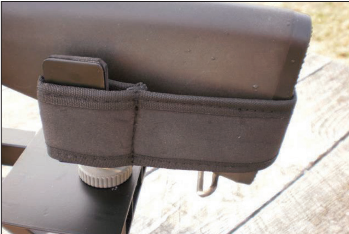
The rest can be used with or without the strap. Place the eyes of the strap over the ears of the yoke.
