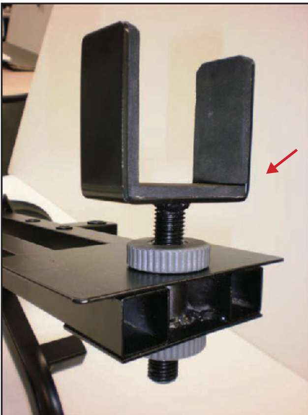
Thread an M-16 locking collar on to the M-16 stem of the yoke, about 3 - 3 ½ inches. Insert the stem through the hole at the rear of the rest. Thread the other locking collar on the stem from the bottom side. Moving the yoke up & down can also be used to adjust elevation.
