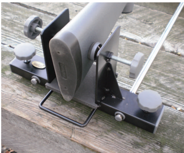
Step 4A: Unload gun and clamp it in vise.
