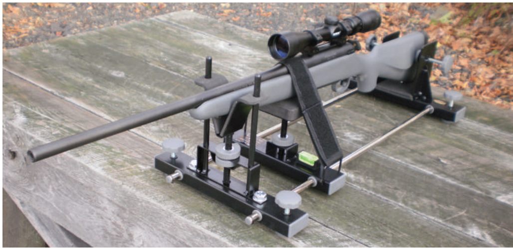
Step 4B: Set the vise in the same location as when you fired. Adjust vise so that reticle is on the + Mark.
