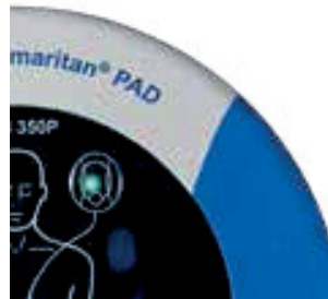
Figure 10. Flashing green LED; no action required.
