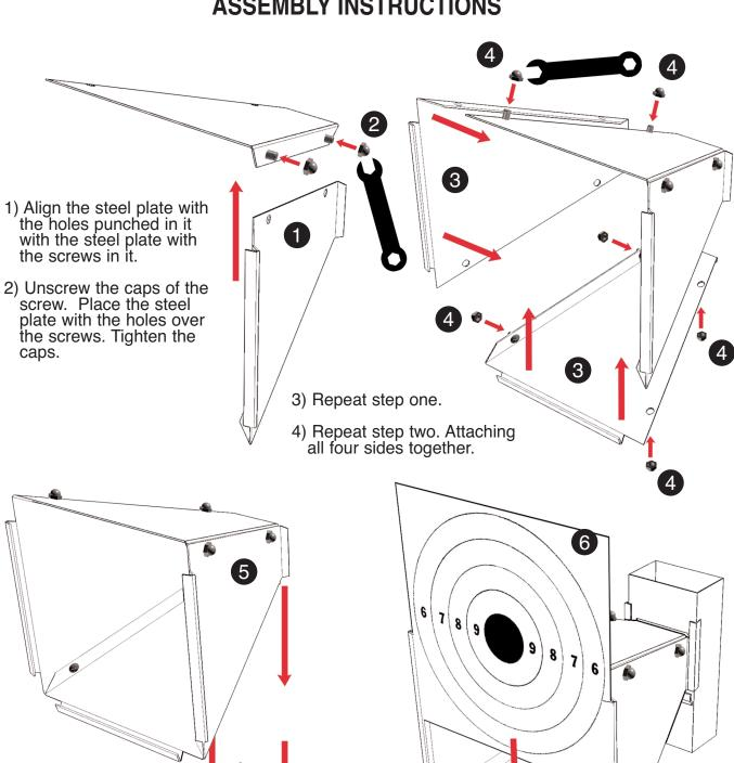
5) Slide fully assembled cone trap into the base.
