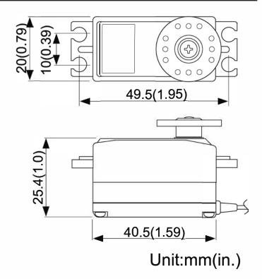
•Use the horn set screw supplied with the servo. (Screw size: 3x8mm) The servo horn can be used the only 3mm in diameter of the hole center.
