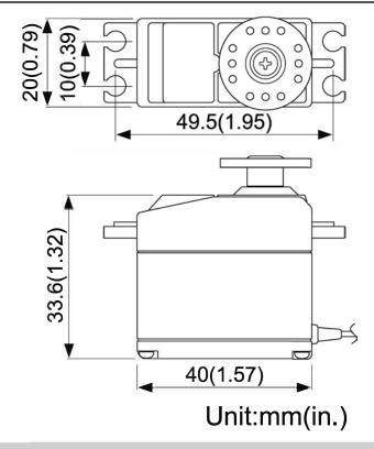
•Use the horn set screw supplied with the servo. (Screw size: 3x8mm) The servo horn can be used the only 3mm in diameter of the hole center.
