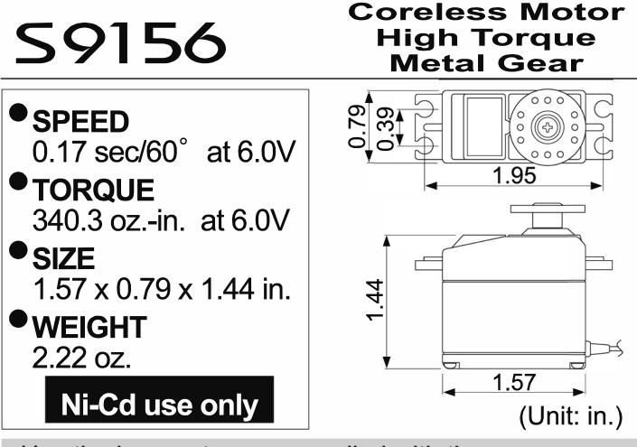
•Use the horn set screw supplied with the servo. (Screw size: 3x8mm) The servo horn can be used the only 3mm in diameter of the hole center.
