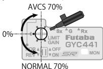
Receiver ON → The GYC441 requires 3-5 seconds to initialize when the power is turned on. Do not move the car and do not move the steering wheel during this initialization or the gyro may not initialize properly. Once the initialization process has been completed, the steering servo wil
