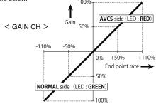
3CH (GAIN CH) is set up with reference to the transmitter manual. Neutral position becomes GAIN 0%. It is divided into AVCS side and NORMAL side. Refer to the GYC441's LED.
