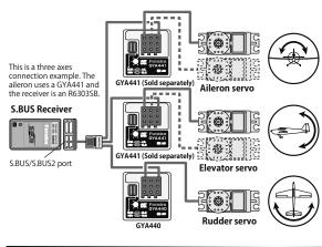
Gyro gain CH(Receiver)←connect→Port2(GYA440)
