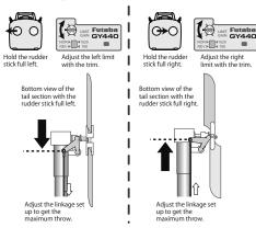
5 If the rudder servo moves to the Right when the nose of the helicopter moves to the Left, the gyro direction is correct. If the rudder servo moves to the Left, switch the direction using the Gyro Direction Switch.
